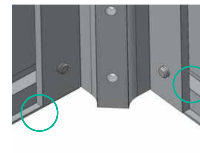
Ring beam lip on the inside inner face
